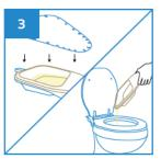
After use, remove the Maxi Slipper Pan Liner with support, place a lid cover over it to contain the odour and sight.
