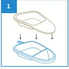
Place the Midi Slipper Pan Liner over the plastic midi slipper pan suppport.
