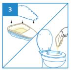
After use, remove the Midi Slipper Pan Liner with support, place a lid cover over it to contain the odour and sight.
